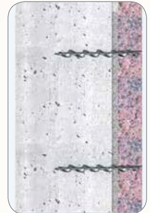
Dimensional Stone to Concrete or Masonry
