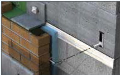
ST-4 Brick relief angle at concrete beam.
