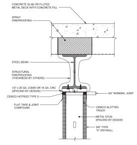
\*NOTE: DOUBLE LAYERS OF 5/8" DRYWALL FOR 2 HOUR FIRE RATING
