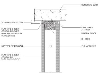
HW-D-0625 1 HR. CONCRETE SLAB
