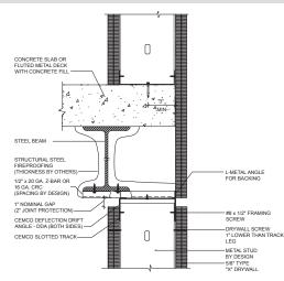
\*NOTE: SINGLE LAYER OF 5/8" TYPE "X" DRYWALL FOR 1 HOUR FIRE RATING, 2 LAYERS FOR 2 HOUR
