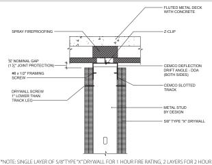
HW-D-0583 Standard Wall Fluted Deck Perpendicular to I-Beam Penetration
