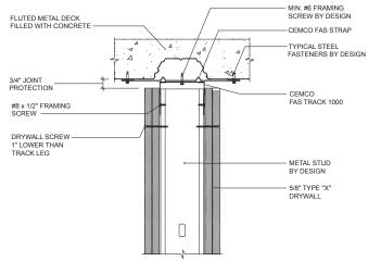
\*NOTE: SINGLE LAYER OF 5/8" TYPE "X" DRYWALL FOR 1 HOUR FIRE RATING, 2 LAYERS FOR 2 HOUR
