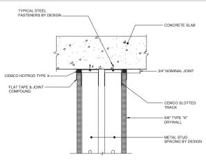
\*NOTE: DOUBLE LAYERS OF 5/8" DRYWALL FOR 2 HOUR FIRE RATING
