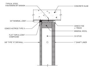
\*NOTE: DOUBLE LAYERS OF 5/8" DRYWALL FOR 2 HOUR FIRE RATING
